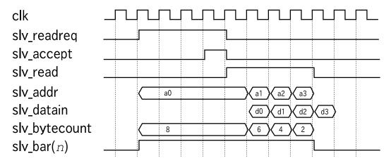
Slave read (GPCle reads from the backend): GPCle requests a read transfer by asserting slv\_readreq. The backend accept the request by asserting slv\_accept when ready. GPCle starts the read transfer immediately after the clock cycle slv\_accept is asserted. The data is transfered from the PCle device to the host computer.
