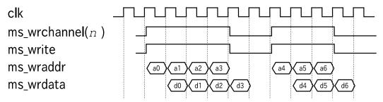
Master write (The backend write to GPCle): The data is transfered from the PCle device to the host computer.
