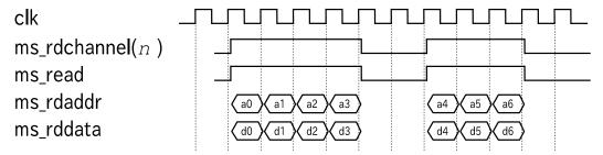
Master read (The backend reads from GPCle): The data is transfered from the host computer to the PCle device.
