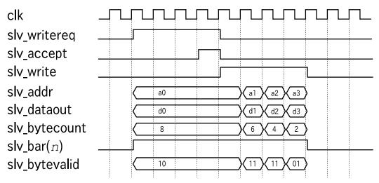
Slave write (GPCle writes to the backend): GPCle requests a write transfer by asserting slv\_writereq. The backend accept the request by asserting slv\_accept when ready. GPCle starts the write transfer immediately after the clock cycle slv\_accept is asserted. The data is transfered from the host computer to the PCle device.
