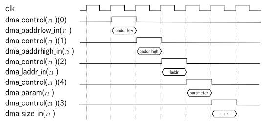
Write to registers of the DMA controller: Set parameters to registers of the DMA controller. The DMA transfer starts when the data size is set by asserting  $dma\_control(n)(3)$ . Here, n denotes channel number of the DMA controller.
